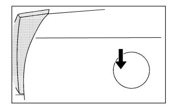
The fuel cap is behind a hinged fuel door on the passenger's side of the vehicle. The fuel door is opened by pushing in on the rear edge until the door pops out.
